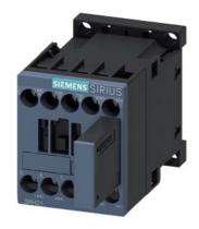
Coupling contactor relay, 2 NO + 2 NC, 24 V DC, 0.85  $\dots$  1.85\* US, with varistor plugged on, Size S00, screw terminal
