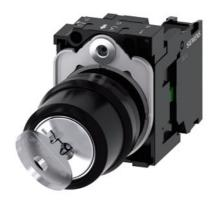
RONIS key-operated switch, 22 mm, round, plastic, Lock No. SB30, with 2 keys, 2 switch positions O-I, latching, 10:30/1:30 o'clock, key removal O+I, with holder, 1NO, screw terminals, possible special locks: SB31, 421, 455, Z=20-unit packaging
