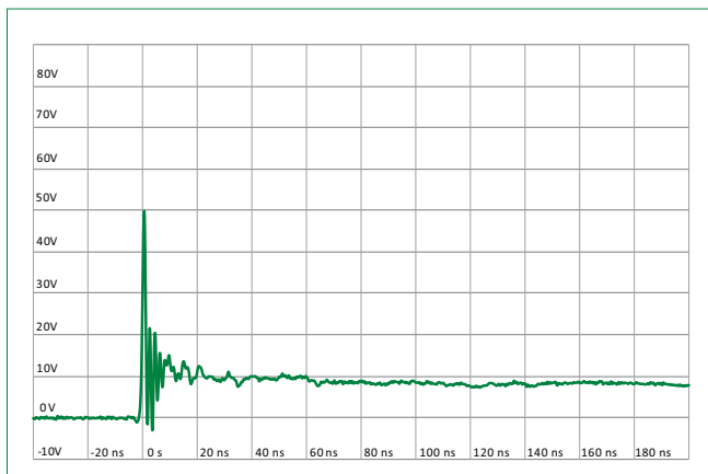
IEC 61000-4-2 +8 kV Contact ESD Clamping Voltage
