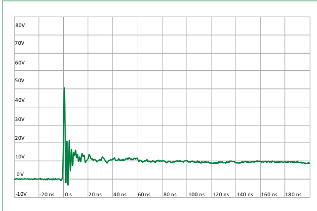
ISO10605 Contact Discharge Plot at +8 kV
