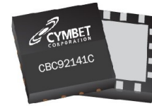
3mm x 3mm x 0.55mm 16-pin MLPQ Package
