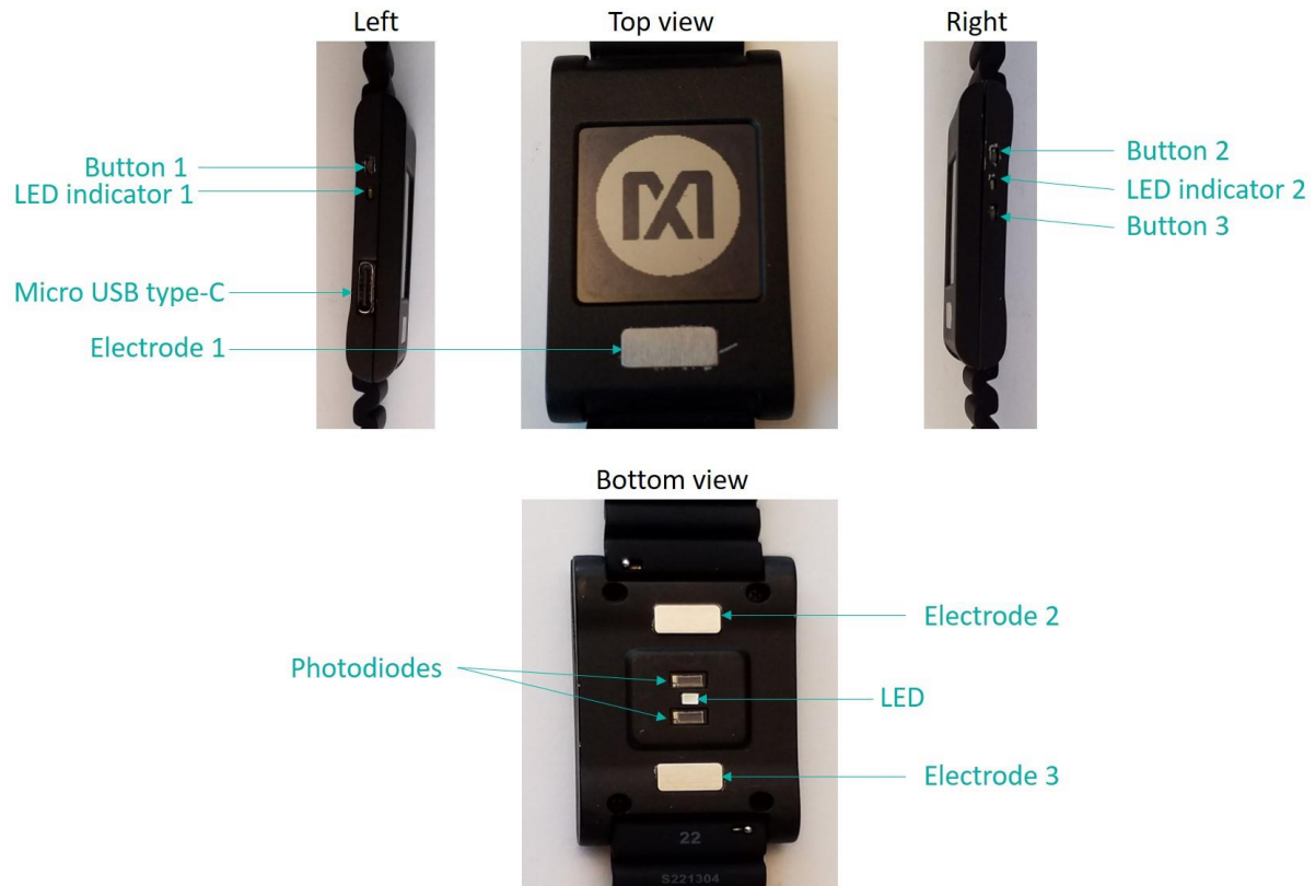
Figure 1. MAXREFDES101# wearable form factor in detail.
