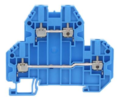
Double-level terminal, Screw connection, Mounting type: Mounting rail TS 35/7.5, Rated cross-section: 2.5 mm<sup>2</sup>, Width: 5.1 mm, Colour: Blue
