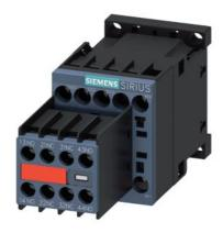
Power contactor, AC-3 9 A, 4 kW / 400 V 2 NO + 2 NC, 24 V DC with diode integrated 3-pole, Size S00 Screw terminal Captive auxiliary switch
