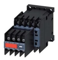
contactor relay, 4 NO + 4 NC, 220 V AC, 50 Hz, 240 V, 60 Hz, size S00, ring cable lug connection, captive auxiliary switch
