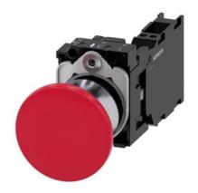
Mushroom pushbutton, 22 mm, round, metal, shiny, red, 40mm, latching, pull-to-unlatch mechanism, with holder, 1 NO+1 NC, spring-type terminal, with laser labeling, lower case
