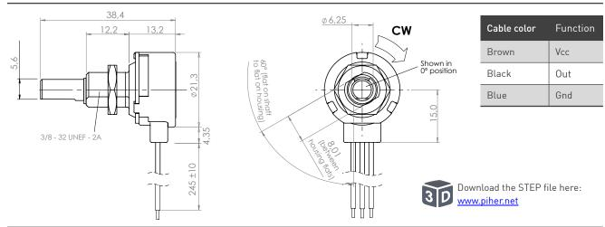
Sensor shipped with one nut installed at base. Assembled washer and extra nut available on request. Other shafts available on request.
