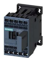
power contactor, AC-3 9 A, 4 kW / 400 V 1 NO, 24 V DC 0.7-1.25\* US, with varistor plugged on, 3-pole, size S00, spring-type terminal not expandable with auxiliary switch
