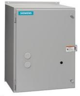
Electrically held lighting contactor, Contactor amp rating 200A, 0 N.C. / 3 N.O. Poles, 208VAC 50/60HZ coil, Non-combination type, (no disconnect device), Encl NEMA type 4X 304 S-Steel, Water/dust tight noncorrosive
