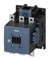
power contactor, AC-3 300 A, 160 kW / 400 V, AC (50-60 Hz) / DC operation 220-240 V AC/DC auxiliary contacts 2 NO + 2 NC 3-pole, frame size S10 busbar connections drive: conventional screw terminal
