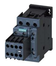
Contactor, AC-3, 15 kW / 400 V, 2 NO + 2 NC, 110 V AC, 50 / 60 Hz, 3-pole, Size S0, screw terminal Removable auxiliary switch
