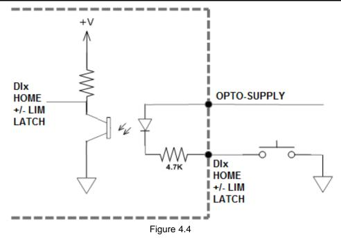
The opto-supply must be connected to +12 to +24VDC in order for the digital inputs, home, limit, and latch to operate.
