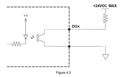
The opto-ground must be connected in order for the digital outputs to operate.
