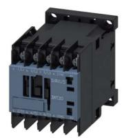
Power contactor, AC-3 9 A, 4 kW / 400 V 1 NC, 400 V AC, 50 Hz 400-440 V, 60 Hz, 3-pole, Size S00, ring cable lug connection
