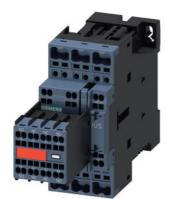
Power contactor, AC-3 12 A, 5.5 kW / 400 V 2 NO + 2 NC, 24 V DC with inserted varistor 3-pole, Size S0 Spring type terminal Captive auxiliary switch
