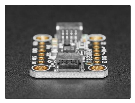
The breakout for the LIS331 family takes one of these little dynamos and puts it on a custom made PCB in the <u>STEMMA QT form factor</u> (), making them easy to interface with. The <u>STEMMA QT connectors</u> () on either side are compatible with the <u>SparkFun</u> <u>Qwiic</u> () I2C connectors. This allows you to make solderless connections between your development board and the LIS331s or to chain them with a wide range of other
