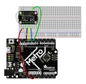
Connect Vin to the power supply, 3V or 5V is fine. Use the same voltage that the microcontroller logic is based off of Connect GND to common power/data ground Connect the SCK pin to Digital #13 but any pin can be used later Connect the SDO pin to Digital #12 but any pin can be used later Connect the SDI pin to Digital #11 but any pin can be used later Connect the CS pin Digital #10 but any pin can be used later
