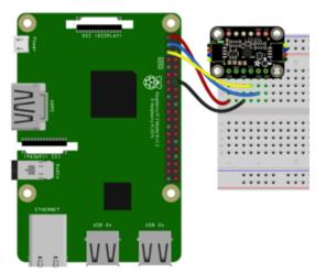
Pi 3V to sensor VCC (red wire) Pi GND to sensor GND (black wire) Pi SCL to sensor SCL (yellow wire) Pi SDA to sensor SDA (blue wire)
