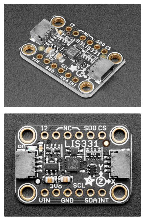
It's not hard to find an accelerometer that can measure accelerations up to 16g, but if you need an accelerometer that can measure even larger amounts of acceleration, your options narrow (The ICM20649 () is a great sensor and can measure up to  $\pm$ 30g).
