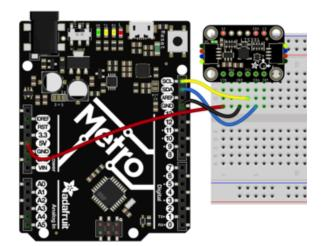
Connect board VIN (red wire) to Arduino 5V if you are running a 5V board Arduino (Uno, etc.). If your board is 3V, connect to that instead. Connect board GND (black wire) to Arduino GND Connect board SCL (yellow wire) to Arduino SCL Connect board SDA (blue wire) to Arduino SDA
