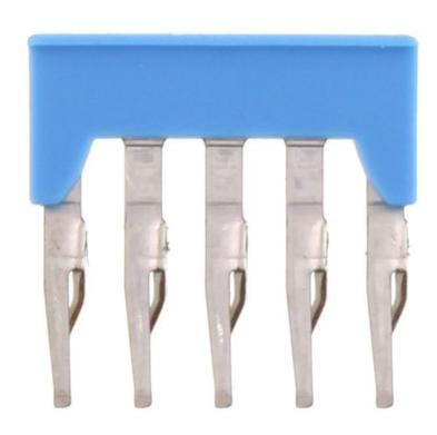
Insulated cross-connector, No. of poles: 5, Mounting type: Plug in, Width: 24.4 mm, Rated cross-section: 2.5 mm², Colour: Blue
