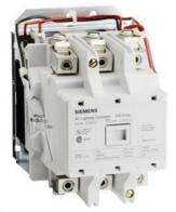
Mechanically held lighting contactor, Contactor amp rating 100A, 0 N.C. / 5 N.O. poles, 24VAC 60HZ coil, Non-combination type, Enclosure NEMA type (open), No enclosure
