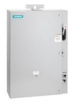
Pump control panel, Size 3, Three phase full voltage, Solid-state overload relay, OLR amp range 25-100A, 24VAC 50-60Hz coil, Standard type contactor, 100A fusible disconnect, 100A/600V fuse clip, HOA Sel Sw. <(>&<)> Start P.B., Enclosure NEMA type 3/3R, Weather proof outdoor use
