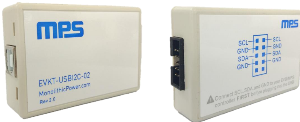
Figure 3: EVKT-USBI2C-02 Communication Interface Device
