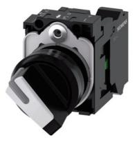
Selector switch, illuminable, 22 mm, round, plastic, white, selector switch, short, 2 switch positions O-I, latching, 10:30h/13:30h, with holder, 1 NO, spring-type terminal, Z=20-unit packaging
