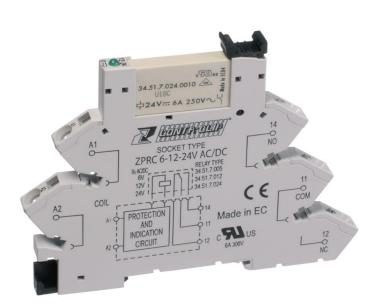
Plug-Relay-Compact (PRC) socket base PRC with tension-spring connection, Mounting type: Mounting rail TS 35, 1 CO contact, Input voltage: 6, 12 or 24 VDC
