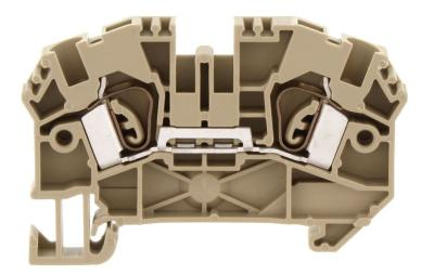
Ex feed-through terminal ATEX-certified, Tension-spring connection, Mounting type: Mounting rail TS 35/7.5, Rated cross-section: 4 mm<sup>2</sup>, Width: 6.1 mm, Colour: Beige
