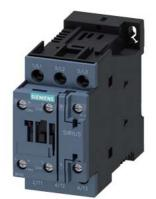
Power contactor, AC-3 32 A, 15 kW / 400 V 1 NO + 1 NC, 125 V DC 3-pole, size S0 screw terminals
