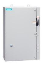
Reversing motor starter, Size 1, Three phase full voltage, Solid-state overload relay, OLR amp range 5.5-22A, 110V 50Hz / 120V 60Hz coil, Combination type, 25A circuit breaker, Encl NEMA type 4X 304 S-Steel, Water/dust tight noncorrosive
