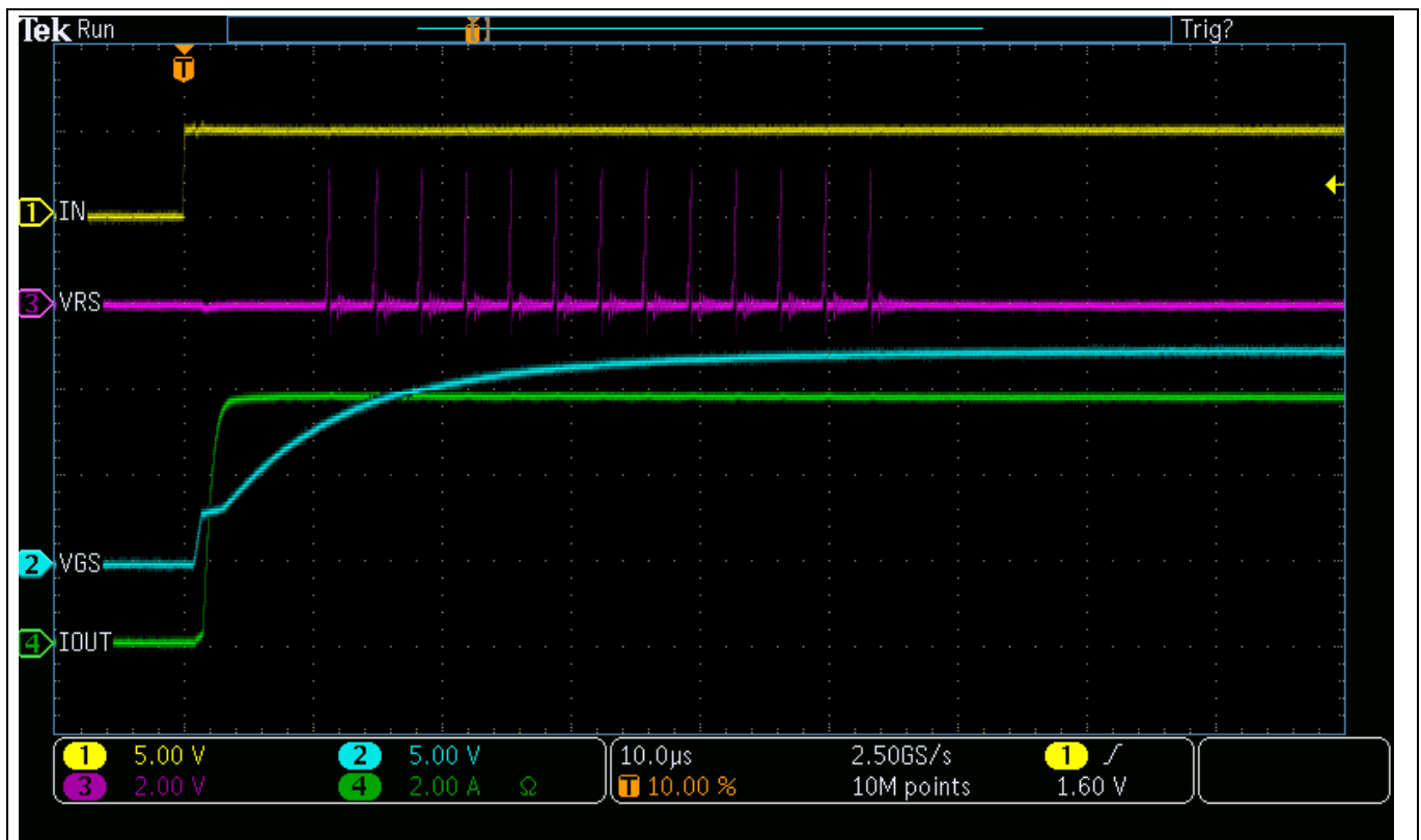
Figure 4 Waveforms from OFF to ON mode [Yellow V_{IN} ; Blue V_{GS(AUIR3241S)} ; Purple V_{RS} ; Green I_{OUT} ]
