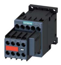
Power contactor, AC-3 9 A, 4 kW / 400 V 2 NO + 2 NC, 230 V AC 50 / 60 Hz, with plugged on varistor, 3-pole, Size S00 Screw terminal Captive auxiliary switch
