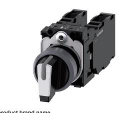
Selector switch, illuminable, 22 mm, round, plastic with metal front ring, white, selector switch, short, 3 switch positions I>O<II, momentary contact type, actuating angle 2x45°, 10:30h/12h/13:30h, with holder, 1 NO+1 NC, 1 NO+1 NC, screw terminal, with laser labeling, upper case and lower case, always upper case at the beginning of the word
