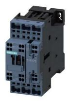
power contactor, AC-3 17 A, 7.5 kW / 400 V 1 NO + 1 NC, 125 V DC with integrated varistor 3-pole, size S0, spring-type terminal suitable for PLC outputs not expandable with auxiliary switch
