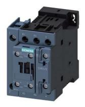
Power contactor, AC-3 25 A, 11 kW / 400 V 2 NO + 2 NC 220 V DC, 50 Hz 4-pole size S0 screw terminals 1 NO + 1 NC integrated
