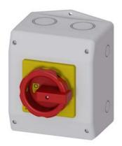
SENTRON, Switch disconnector 3LD, emergency switching-off switch, 6-pole, lu: 25 A, operating power / at AC-23 A 400 V: 9.5 kW, Molded plastic encapsulation for metric cable gland, 1 NC, 1 NO, rotary operating mechanism, red/yellow
