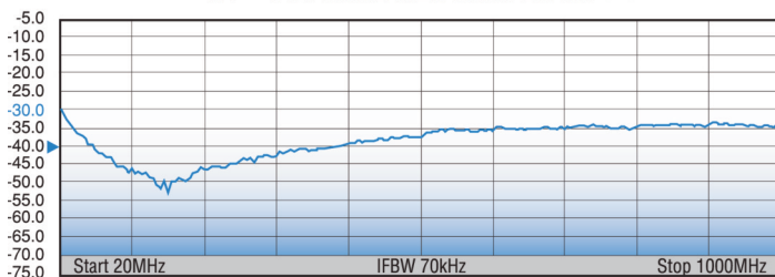
S11 TYPICAL RETURN LOSS (dB)
