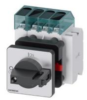
Load disconnector 3LD3, lu 16 A Main switch 3-pole + N Rated operating capacity at AC-23 A at 400V 7.5kW Front plate mounting Basic switch with Central hole mounting 22.5mm Toggle drive black 48x48 mm with auxiliary switch 10E + 1S
