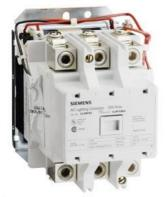
Mechanically held lighting contactor, Contactor amp rating 200A, 0 N.C. / 3 N.O. poles, 208VAC 60HZ coil, Non-combination type, Enclosure NEMA type (open), No enclosure
