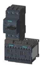
FUSELESS LOAD FEEDER REVERSING OPERATION, AC 400V, S00 2.8. . .4A, AC 110/120V 50/60HZ SCREW TERMINAL FOR RAIL MOUNTING, TYPE OF ASSIGNMENT 2,IQ = 150KA (ALSO FULFILLS TYPE OF ASSIGNMENT 1) 1NC (CONTACTOR)
