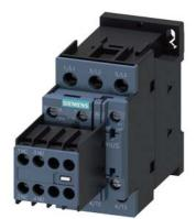
power contactor, AC-3 25 A, 11 kW / 400 V 2 NO + 2 NC, 220 V AC, 50 / 60 Hz, 3-pole, Size S0, screw terminal Removable auxiliary switch
