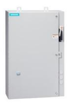
Non-reversing motor starter, Size 3, Three phase full voltage, Solid-state overload relay, OLR amp range 25-100A, Combination type, 125A circuit breaker, Enclosure NEMA type 4/12, Water/dust tight for outdoors, Standard width enclosure
