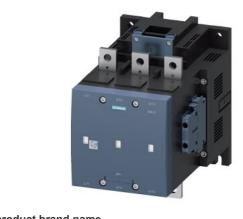
vacuum contactor, AC-3 400 A, 200 kW / 400 V AC (50-60 Hz) / DC operation 575-600 V AC/DC auxiliary contacts 2 NO + 2 NC 3-pole, frame size S12 busbar connections drive: conventional
