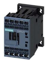
power contactor, AC-3 12 A, 5.5 kW / 400 V 1 NC, 48 V DC, with diode integrated, 3-pole Size S00, Spring-type terminal
