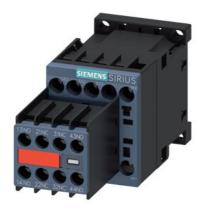
Power contactor, AC-3 7 A, 3 kW / 400 V 2 NO + 2 NC, 24 V DC 3-pole, Size S00 Screw terminal Auxiliary switch block permanently mounted
