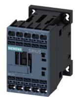
Contactor, 2NO + 2NC, AC-3, 5.5 kW, 110 V AC, 50 Hz, 120 V, 60Hz, 4-pole, 2NO + 2NC, Size S00, Spring-type terminal
