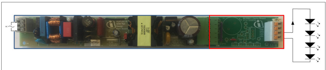
Figure 7 XDPL8218 BCR601 system - top side
