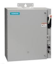
Pump control panel, Size 1, Three phase full voltage, Solid-state overload relay, OLR amp range 5.5-22A, 190-220/220-240V 50/60Hz coil, Standard type contactor, 30A fusible disconnect, 30A/600V fuse clip, HOA Sel Sw. <(>&<)> Start P.B., Enclosure NEMA type 3/3R, Weather proof outdoor use
