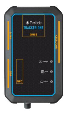
As the GNSS antenna faces the top of the case, you also want the top of the case facing the sky to the greatest extent possible. You will likely be be unable to get a GNSS lock with the top facing down.
