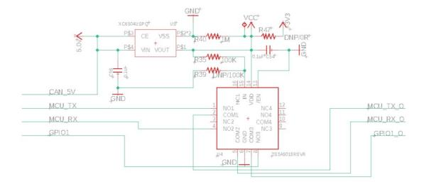
Because this is an analog switch, the nRF52840 current limitations, 2 mA in standard drive (the default), and 9 mA in high drive also apply on the M8 side of the analog switch. The switch is rated up to 300 MHz, higher than the highest UART or I2C baud rate. The 3.3V recommended maximum for GPIO also applies on the M8 connector.
