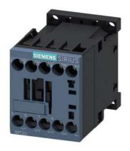
power contactor, AC-3 12 A, 5.5 kW / 400 V 1 NC, 24 V DC 0.7-1.25\*US with integrated diode, 3-pole size S00, screw terminal suitable for PLC outputs not expandable with auxiliary switch
