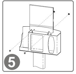
To mount the MP-075 Sign Holder, align the holes of the holder with the holes of the dispenser. With a flathead screwdriver, attach using (2x) barrel screws included with sign holder.
