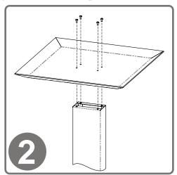
Use Phillips screwdriver to secure base to column with (4x) screws (10-32 x 5/16").
