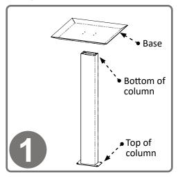
To secure base to column, turn column upside down (with top plate down) and place base inverted, as shown, on column.
