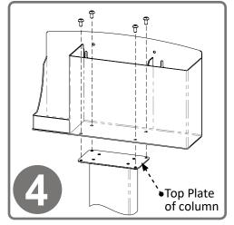
Attach the RS001-0212 Respiratory Hygiene Station to the column using (4x) screws included with stand. Tighten.
