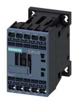
Contactor relay, 2 NO + 2 NC, 220 V AC, 50 / 60 Hz, Size S00, Spring-type terminal
