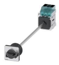
Load disconnector 3LD3, lu 25 A Main switch 3-pole Rated operating capacity at AC-23 A at 400V 9.0kW floor mounting Basic switch with door coupling Central hole mounting 22.5mm Toggle drive black 48x48 mm with auxiliary switch 1OE + 1S
